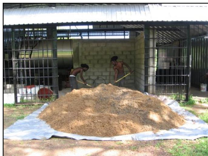
In this photo you can see the boiler and the cooker arranged in the plant. Walls are provided to segregate different functions such as the boiler room and the processing room. Especially important is the wall between the incoming feedstock and the final product. Industry standards provide that workers in one section do not cross into the other section thereby preventing contamination.
